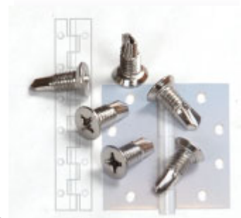
Special Hinge Screws — Self drilling, self tapping, #14 screw with #12 head to replace #12 stripped out hinge screws
